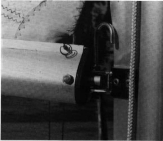
Photo 23 Connect boom to mast
