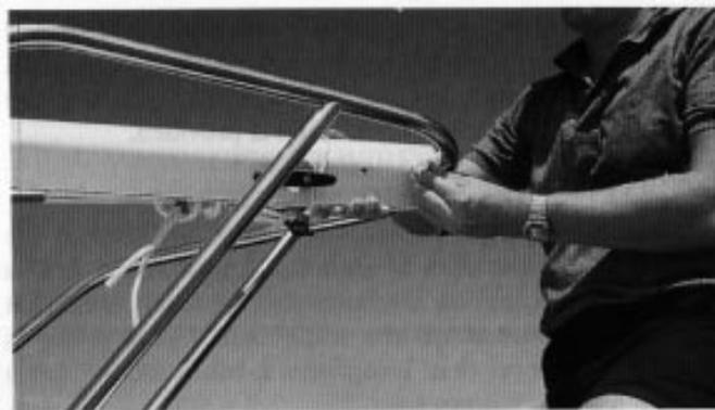
Photo 11 Mast bolted to front rail
