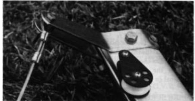
Photo 2 Rear mast support wire attachment (backstay)
