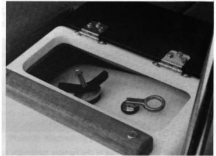
Photo 22. Water Valve and air vent.
