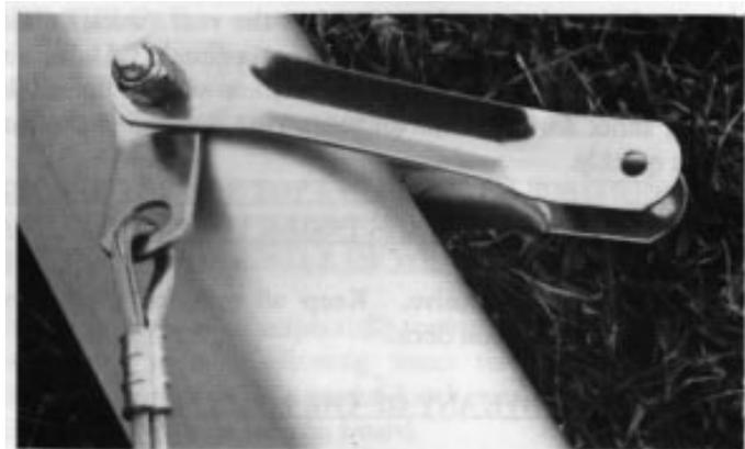
Photo 3 Top side support wires (upper shrouds)
