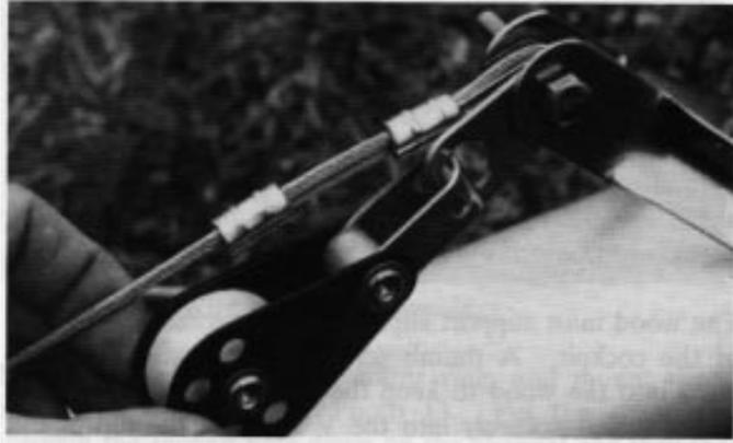
Photo 4 Forward mast support wire and jib pulley
